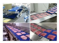
Our loading systems, upon receiving portions from slicers, can automatically re-arrange them into the precise pattern requested by the thermoforming machine, thanks to diverting, aligning, and accelerating modules.
